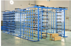
无柱积极传动筒子架 None pillar positive drive creel
