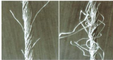
紧密纱线和环锭纱对比图片 Compact Spun yarn vs. ring spun yarn
